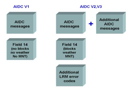
The diagram shows that everything in AIDC Version 1 is included in AIDC V2 and V3. As such, an AIDC V1 ATS Unit is interoperable with an AIDC V2 or 3 ATS Unit.
